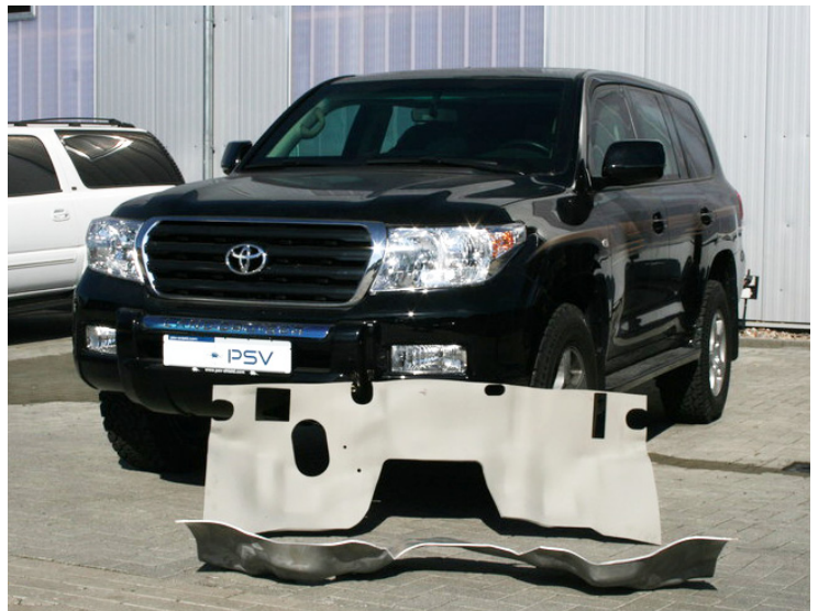
▲ Firewall (hardness 600 HB) for a Toyota Land Cruiser.
