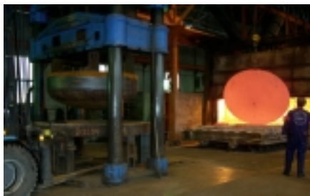
The picture sequence shows a pressure vessel head being made of a compound plate.
