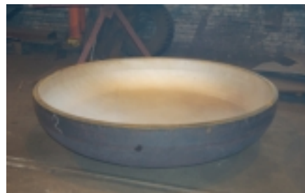
The picture sequence shows a pressure vessel head being made of a compound plate.
