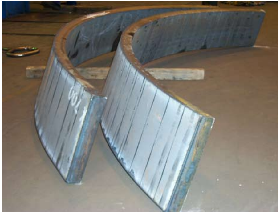
Formed cone segments – four segments make a complete cone
