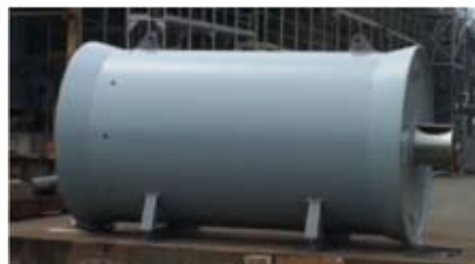
Complete support roller prior to installation
