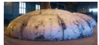
Two segmented pressure vessel heads ready for delivery to Chile
