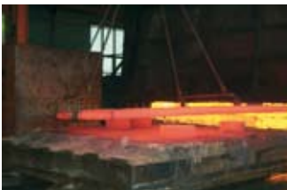
Hot forming of 105 mm thick plate (pictures 1 – 6)
