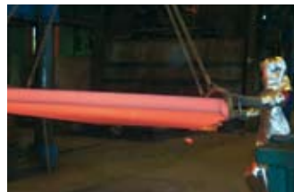
Hot forming of 105 mm thick plate (pictures 1 – 6)
