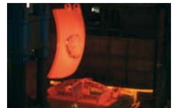
Solution heat treatment after hot forming (pictures 7 – 8)
