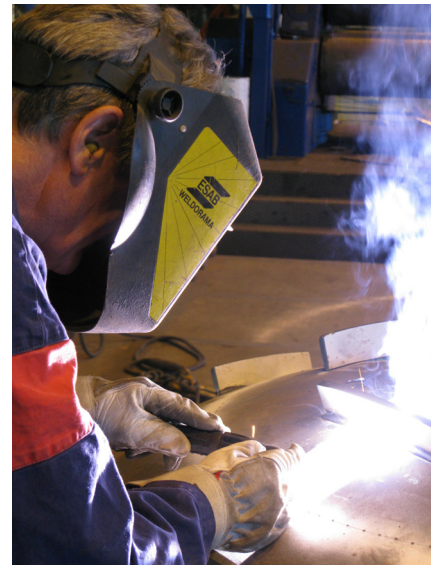
Welding of assembly details on detonation chamber.
