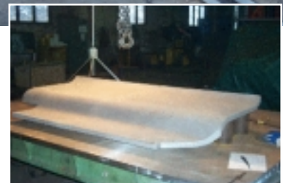
Two examples of protection plates in thicknesses 14,5 and 35 mm, delivered in over 1000 individuals.
