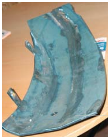
Pressure vessel head pressed and subjected to ballistic testing by Deform
