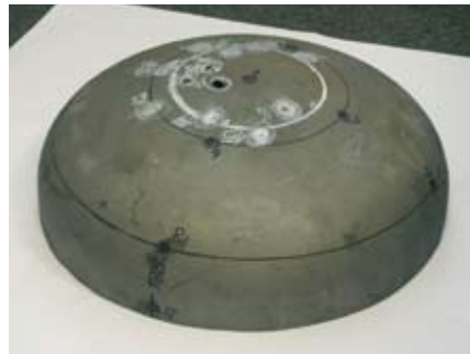
Pressure vessel head pressed and subjected to ballistic testing by Deform
