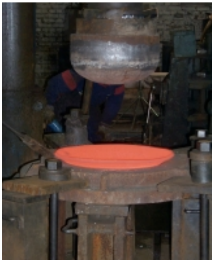
Pre-formed circular blank on the press.
