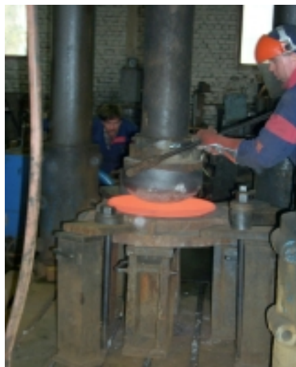
Adjusting the position of the blank.
