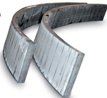
Formed cone segments – four segments make a complete cone.
