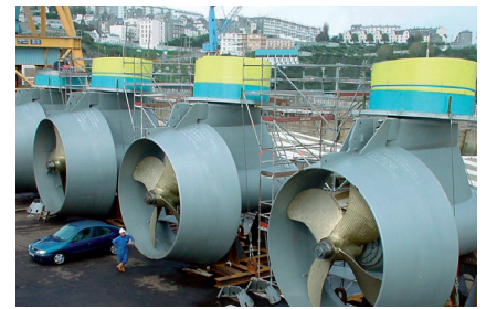
Finished pod housing on the quay for loading.
