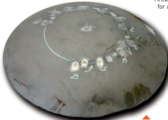
▲ We use ballistic tests to evaluate our formed products. Test shooting has taken place in, for example, Germany, France and Sweden.
