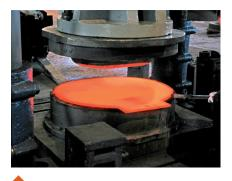
Hot forming of protection plate in quenched and tempered steel.
