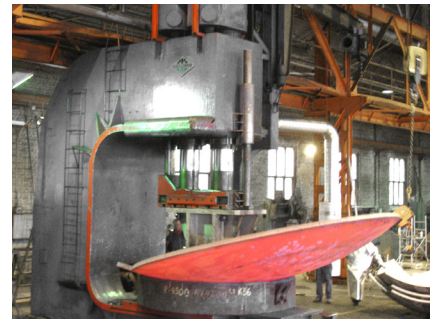
3D-forming of a crown plate with a diameter corresponding 4200 mm.
