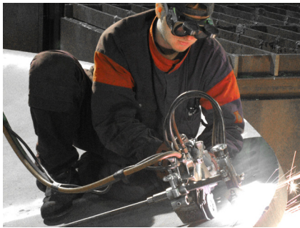
3D-cutting of a bevel on a formed crown plate.
