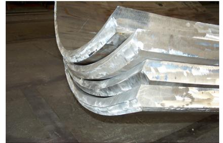
Patrik Molin in front of a test assembled 2:1 segmented head of 12.5 metres in diameter. The head comprised 26 different parts and the plates were 52 mm thick 2205 (1.4462). Cold forming was used throughout. The perfect fit illustrates our customary superb quality.
