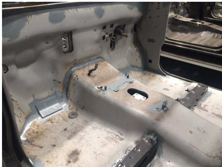
▲ A customer unique solution on a floor and firewall. Notice how well the sheet follows the shape of the vehicle and the minimal remaining welding.
