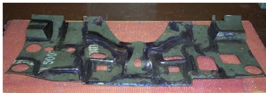
▲ Picture above shows a traditionally manufactured firewall in multiple, overlapping and welded plates.
