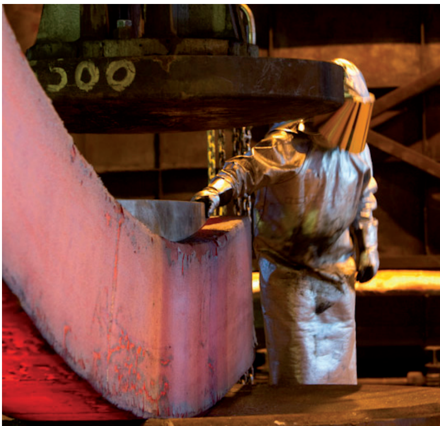
▲ Six segments together form a circular bearing with a nine-metre diameter. Such bearings are used in large slewing cranes. The end customer is German.
