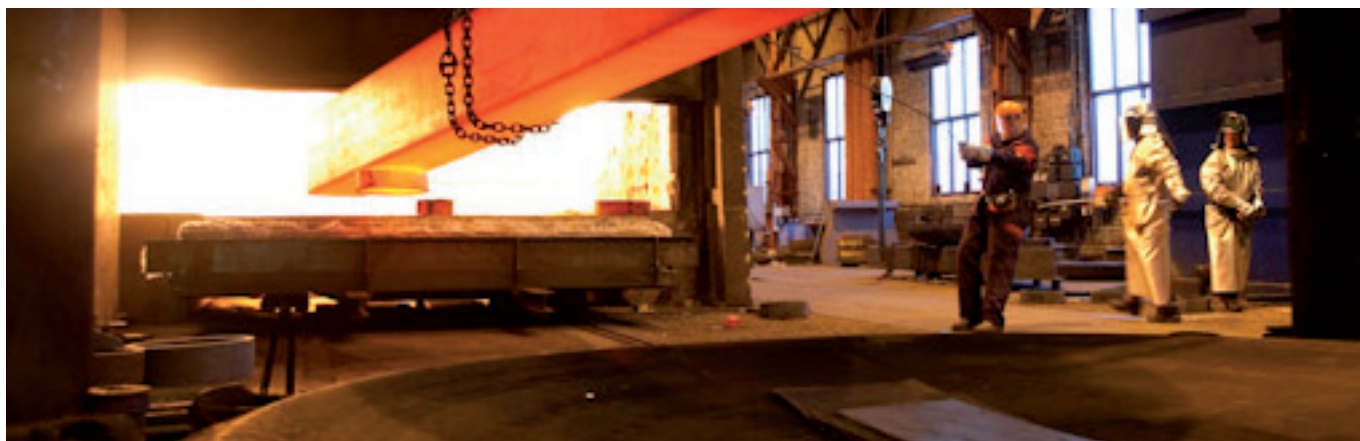
▲ Heating a segment before forming.
